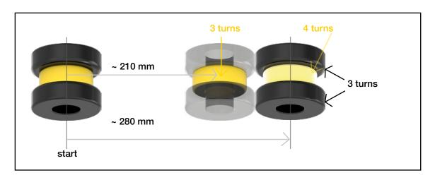
But it doesn't stop at that: Fine tuning is also possible by using additional support wheels - normally in the upper part of the tool. Warpage will also be decreased with this method.
