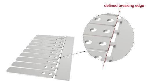
As shown in the picture, a metal strip (carrier plate) was produced on a side with a connection bridge to the single part. You see that it is also important to use the 3-side macro-joint connection.
