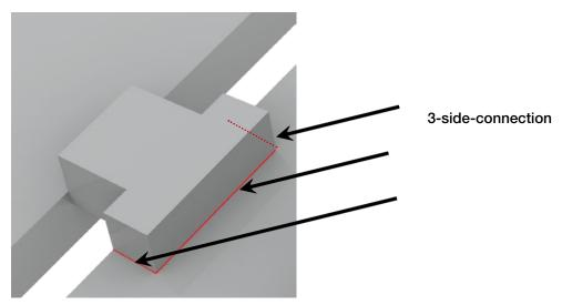
The machine operator does not have to worry about that the connection bridges create burrs that can fall into the brush table and cause scratches on the proceeding processes.
