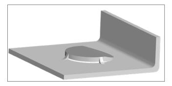
• The connections made by production of the knock-out feature a very high sharp-edged burr when breaking out the slug. This can damage the cable at time of assemble.
